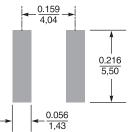
\* For optional tin-lead and tin-silvercopper terminations, dimensions are for the mounted part. Dimensions before mounting can be an additional 0.005 inch / 0.13 mm.
