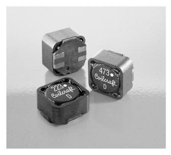
The MSC1278 coupled inductors are designed with high leakage inductance for use in SEPIC applications. The loosely coupled windings (K  $\approx$  0.8) improve SEPIC efficiency by reducing circulating current and provide twice the ripple current reduction of separate inductors.
