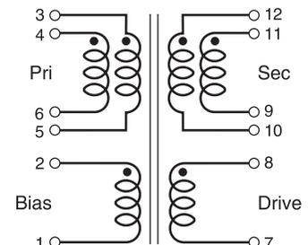
Primary windings and secondary windings to be connected in parallel on PCB board
