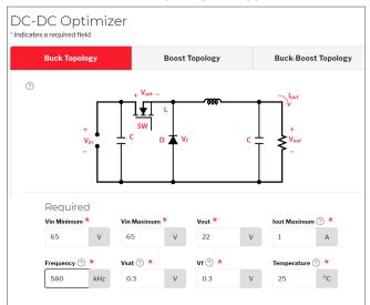
Note the input voltage as well as the output current and voltage are specified as part of the design requirement. The switching frequency may represent some design freedom if a driver IC is not yet selected, but generally the only degree of freedom in selecting the inductor value is the amount of ripple current to be allowed.
