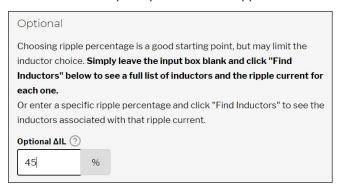
From these inputs, the Coilcraft **DC-DC Optimizer** tool calculates the resulting ripple current for each inductor in the tool within a range of the entered ripple current.
