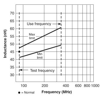
Figure 2. Tolerance change with frequency for an inductor
