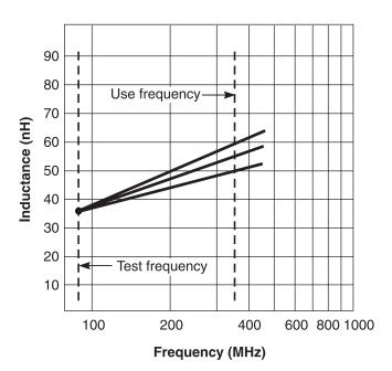
Figure 1. Inductance change with frequency for three different inductors
