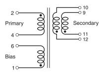
Secondary windings to be connected in parallel on PC board
