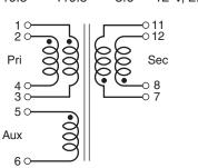
These pins to be connected on the PC board: 1 to 2, 3 to 4, 7 to 8 and 11 to 12.
