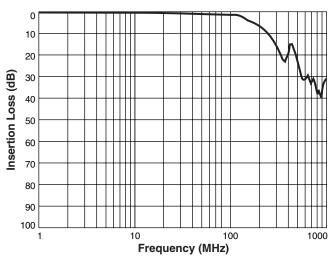
802.3af specification: 1.0 min dB from 0.1 MHz to 100 MHz 1.2 min dB at 125 MHz
