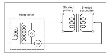
computing. Because magnetic components can be used in multiple applications involving different hazard levels, the hipot test voltage for any specific application must be carefully determined by referring to the pertinent standards for the equipment type.
