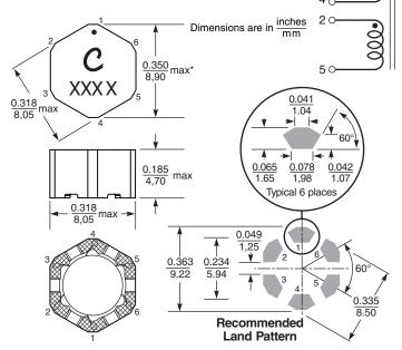
\* Dimensions are of the case not including the termination. For maximum overall dimensions including the termination, add 0.005 in / 0,13 mm. For optional tin-lead and tin-silver-copper terminations, dimensions are for the mounted part. Dimensions before mounting can be an additional 0.005 inch / 0,13 mm).
