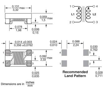
The PFD3215 has a footprint less than  $3.2 \times 2.3$  mm, making this shielded coupled inductor ideal for applications with limited board space. It is designed for use in a variety of circuits including flyback, multi-output buck, SEPIC and Zeta.
