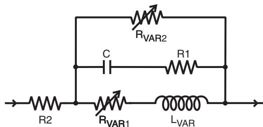
The value of the frequency-dependent variable resistor  $R_{VAR1}$  is calculated from:
