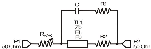
Each model should only be analyzed at the input and output ports. Individual elements of the model are not determined by parameter measurement. The elements are determined by the overall performance of the lumped element model compared to the measurements of the component.
