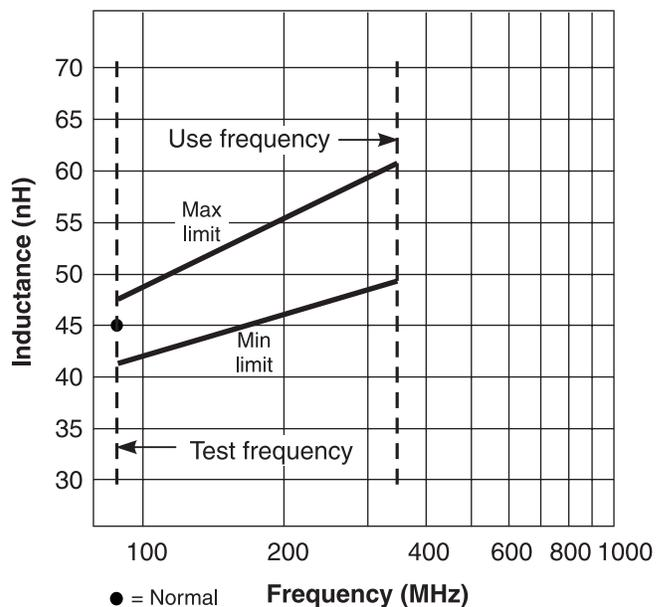
Figure 2. Tolerance change with frequency for an inductor
