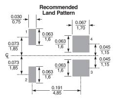
Dimensions are in  $\frac{\text{inches}}{\text{mm}}$
