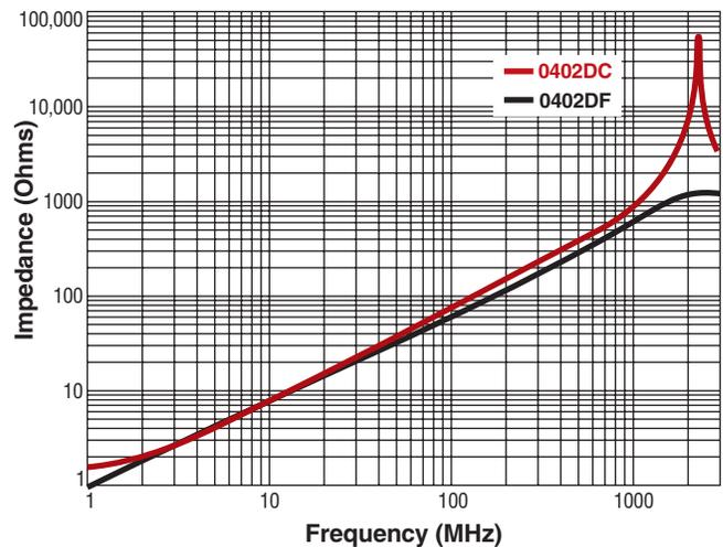
Figure 1. Coilcraft 0402DC & 0402DF 120 nH Impedance
