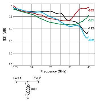
Figure 3. Broadband Conical Inductors
