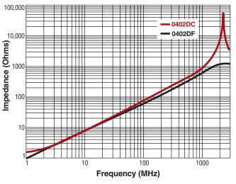
Figure 1. Coilcraft 0402DC & 0402DF 120 nH Impedance
