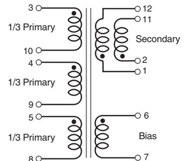
Primary windings to be connected in series on the PC board. Secondary winding to be connected in parallel on the PC board.
