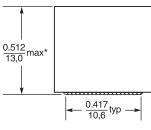
\* For optional tin-lead and tin-silvercopper terminations, dimensions are for the mounted part. Dimensions before mounting can be an additional 0.005 inch / 0,13 mm
