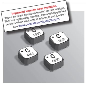
The LPD5030 coupled miniature shielded inductors are only 3 mm high and 5 mm square. They are ideal for use in a variety of circuits including flyback, multi-output buck and SEPIC.
