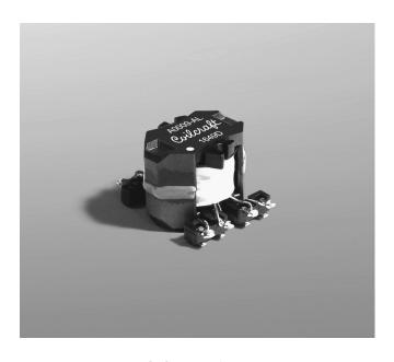
This surface mount flyback transformer is designed for use with Texas Instruments LM5000 DC/DC regulator. The core completely encloses the windings to minimize EMI interference. The transformer features very low DCR. 500 Vrms isolation and a leakage inductance rating of just 1.0 µH. Coilcraft can also custom engineer a transformer to meet your specific requirements.
