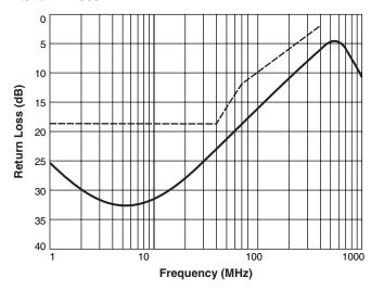
802.3at specification: 18 dB min from 1 MHz to 40 MHz 16 dB min at 50 MHz 12 dB min at 80 MHz 10 dB min at 100 MHz
