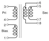
Secondary windings to be connected in parallel on the PC board
