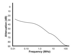
Figure 1. Ideal frequency response predicted for second order filter with Coilcraft E3493 common mode inductor and 0.005 µF capacitors.
