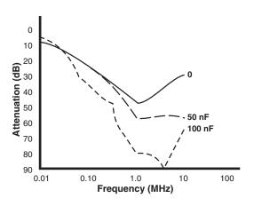
Figure 6. Frequency response of a 2nd order filter with Coilcraft E3495 for various capacitor values.
