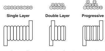
Figure 4. The three winding configurations examined
