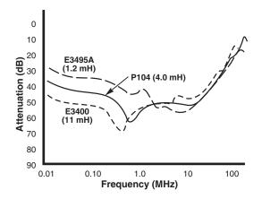
Figure 10. Common mode attenuation of second order filters with 0.005 µF capacitors and various E core inductors.
