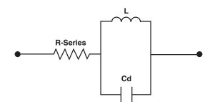
Figure 3. Model of an inductor (one common mode inductor winding).
