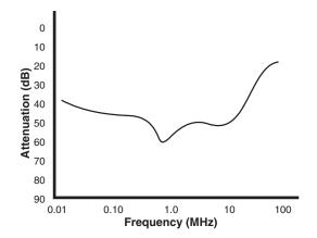
Figure 2. Measured frequency response of second order filter with Coilcraft E3493 common mode inductor and 0.005 µF capacitors.
