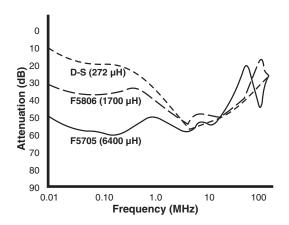
Figure 9. Common mode attenuation of second order filters with 0.005 μF capacitors and various toroid inductors.
