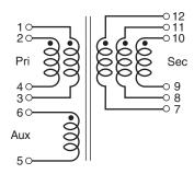
Primary windings and secondary windings to be connected in parallel on the PC board.
