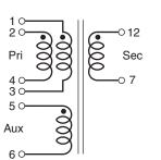
The primary windings to be connected in parallel on the PC board.
