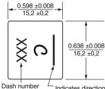
Indicates direction of terminals and start (short) lead. Connect high dv/dt here for lowest EMI.
