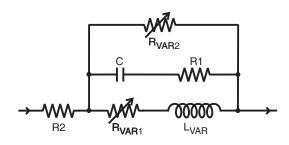
The value of the frequency-dependent variable resistor R<sub>VAR1</sub> is calculated from:
