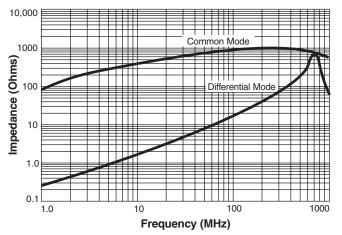
\* Measured on HP 8753D network analyzer. Ref: 50 Ohms.
