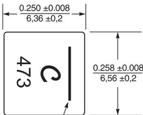
Indicates direction of terminals and start (short) lead. Connect high dv/dt here for lowest EMI.
