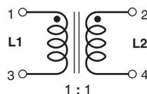
The MSC1278 coupled inductors are designed with high leakage inductance for use in SEPIC applications. The loosely coupled windings ( $K \approx 0.8$ ) improve SEPIC efficiency by reducing circulating current and provide twice the ripple current reduction of separate inductors.
