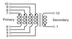
Primary windings to be connected in parallel on PC board
