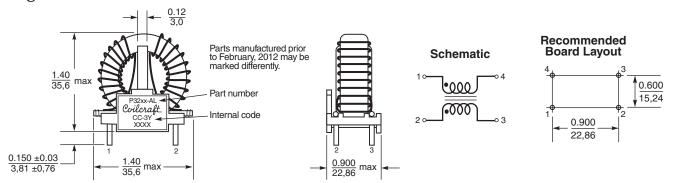
Terminations: Tin-silver over copper; #16 AWG (0.051"/1,29 mm). #16 AWG tinned copper wire leads except P3223-A, which has #18 AWG leads.
