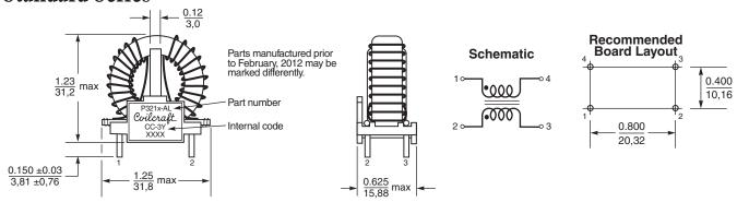
Terminations: Tin-silver over copper; #16 AWG (0.051"/1,29 mm) except P3217-A, which has #18 AWG (0.040"/1.02 mm).
