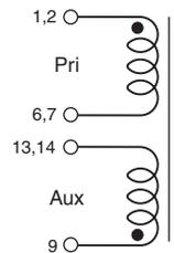
The windings are connected internally as shown
