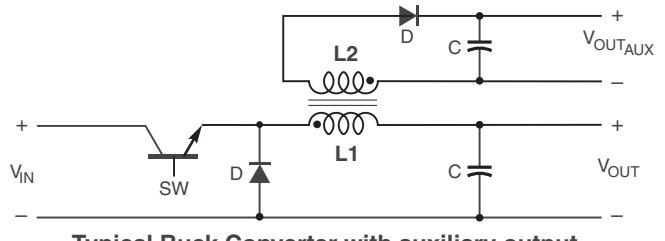
Typical Buck Converter with auxiliary output
